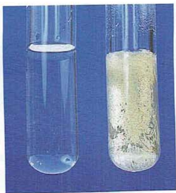
Figure 18.02 The silver mirror formed when Tollens' reagent is warmed with an aldehyde.
