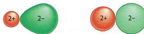
Figure 19.03 Ion polarisation: a small highly charged cation can distort the shape of the anion but a larger cation cannot
